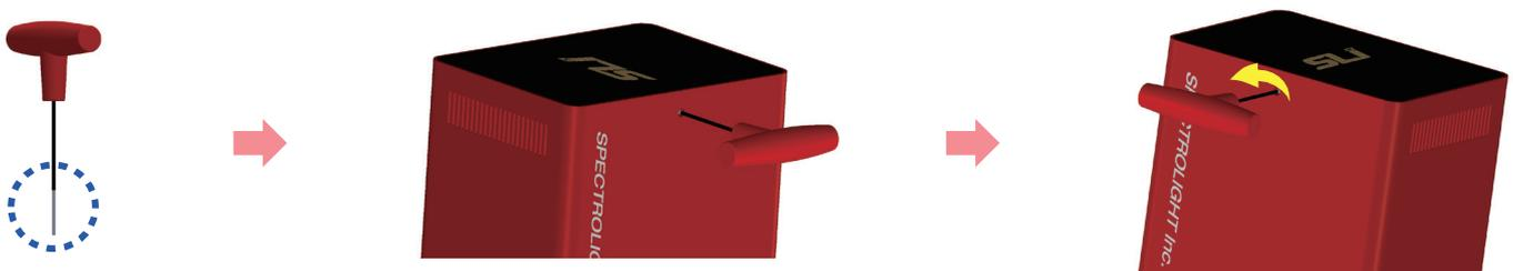
Insert the T-Wrench into the hole until the **SILVER SECTION** of the wrench is **INSERTED ALL THE WAY** inside the hole. Afterwards, turn the wrench **COUNTER CLOCKWISE** (to the left) around a few times as shown in the figure above.
