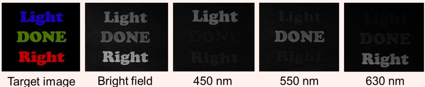
Figure 2. The image of the whole target (left), the brightfield image (2nd image), and the hyperspectral images obtained with three different wavelengths (3rd ~ 5th images).
