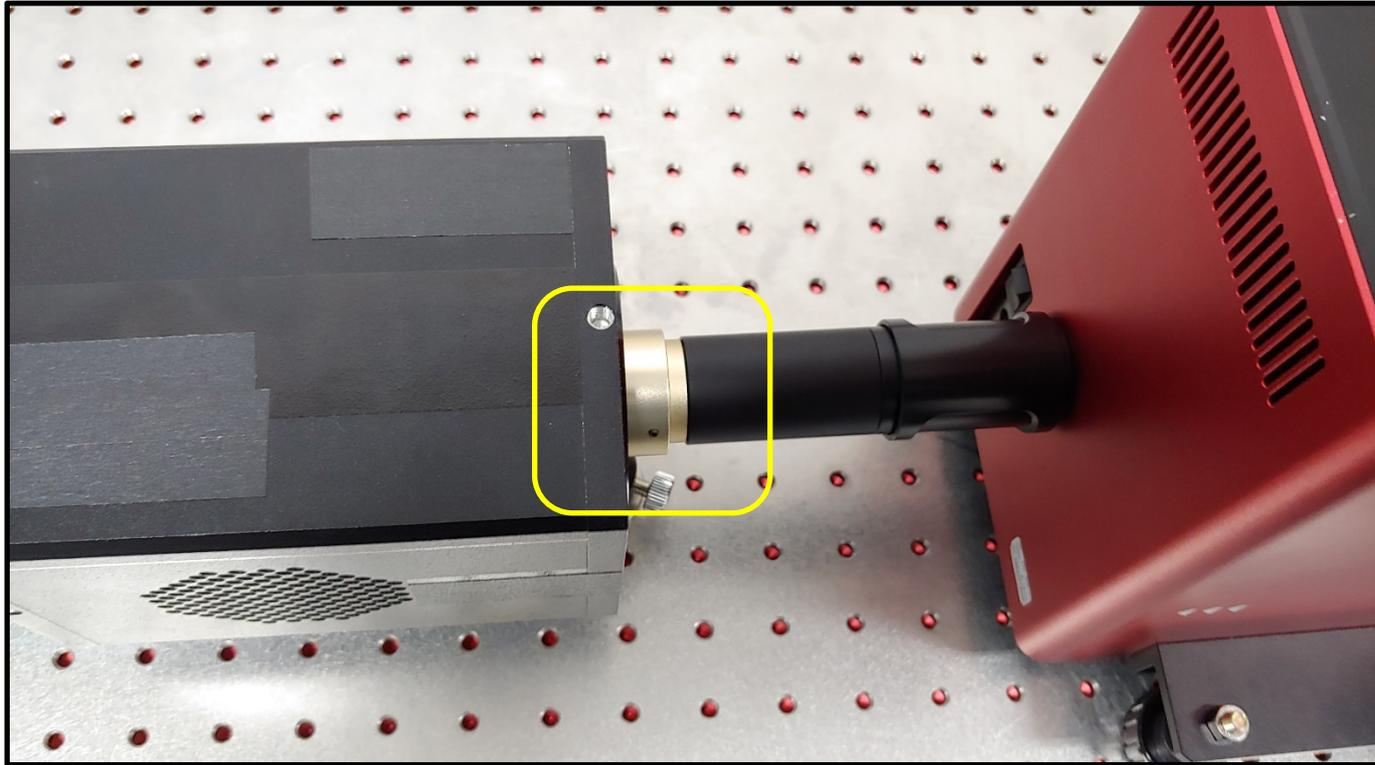
Assemble the c-mount gold adapter to the gold adapter.
