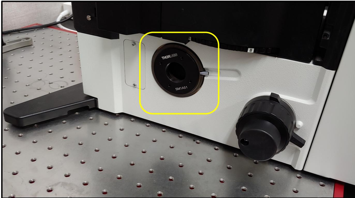
Next, attach the **emission port adapter** for attaching lens tube. The adapter is available for different types of commercial microscopes.
