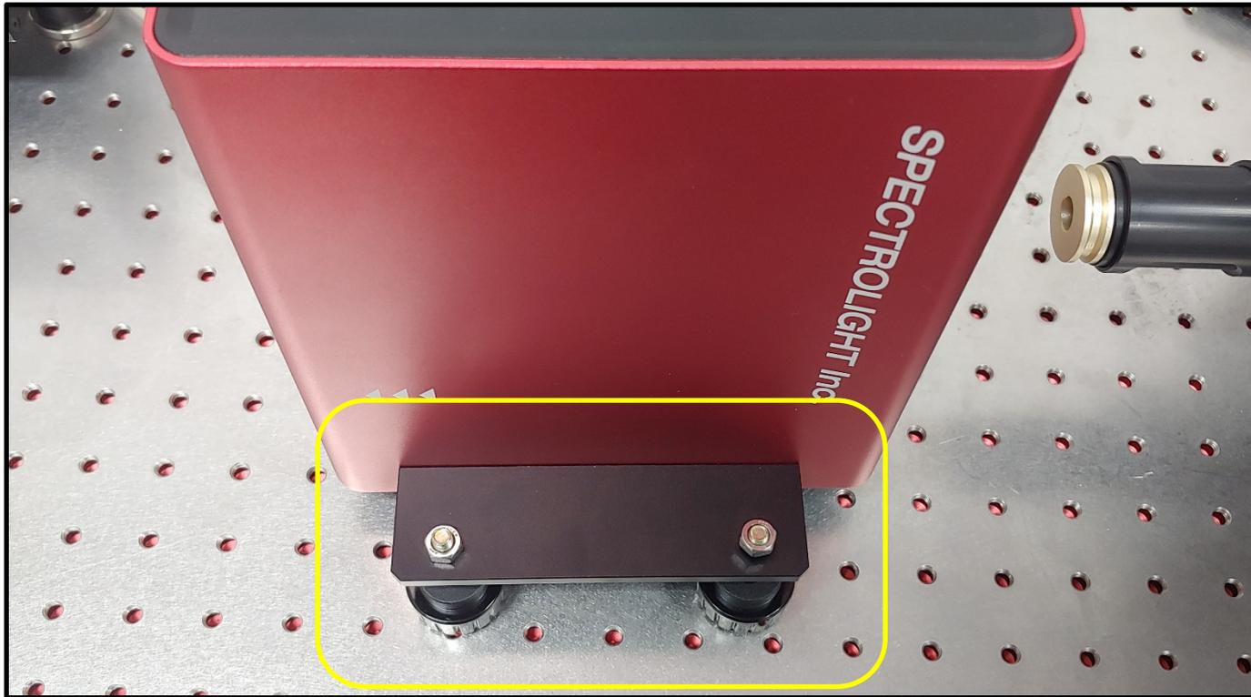
Place FWS Poly on the provided **height adjustable platform** for FWS Poly. The **screws** can be used to adjust the balance and height of FWS Poly.
