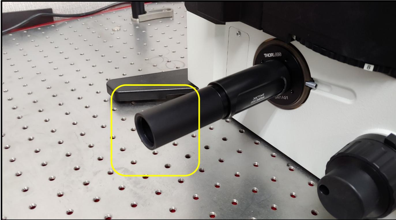
Then, screw in the second lens tube. The length of this tube is about 3 inches.
