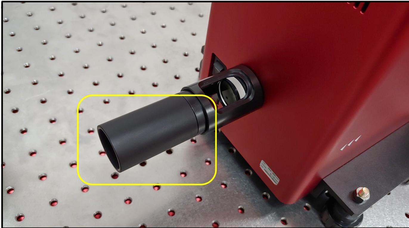
Attach the last **lens tube**. This lens tube doesn't contain any lens and is about 3 inches long.
