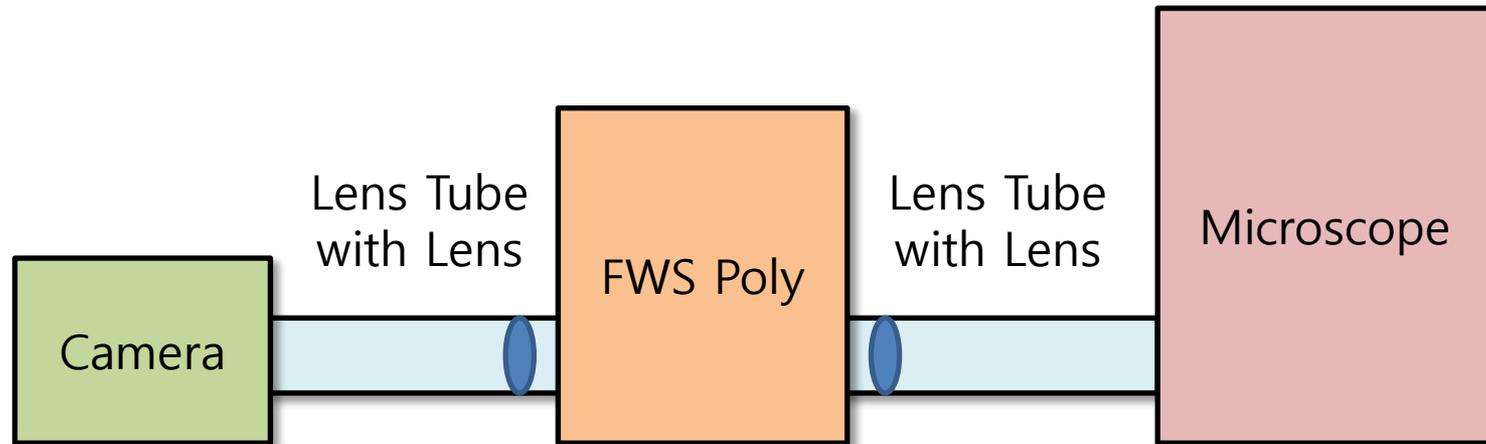
Here is a schematic diagram to show the overall assembly of FWS Poly to microscope.
