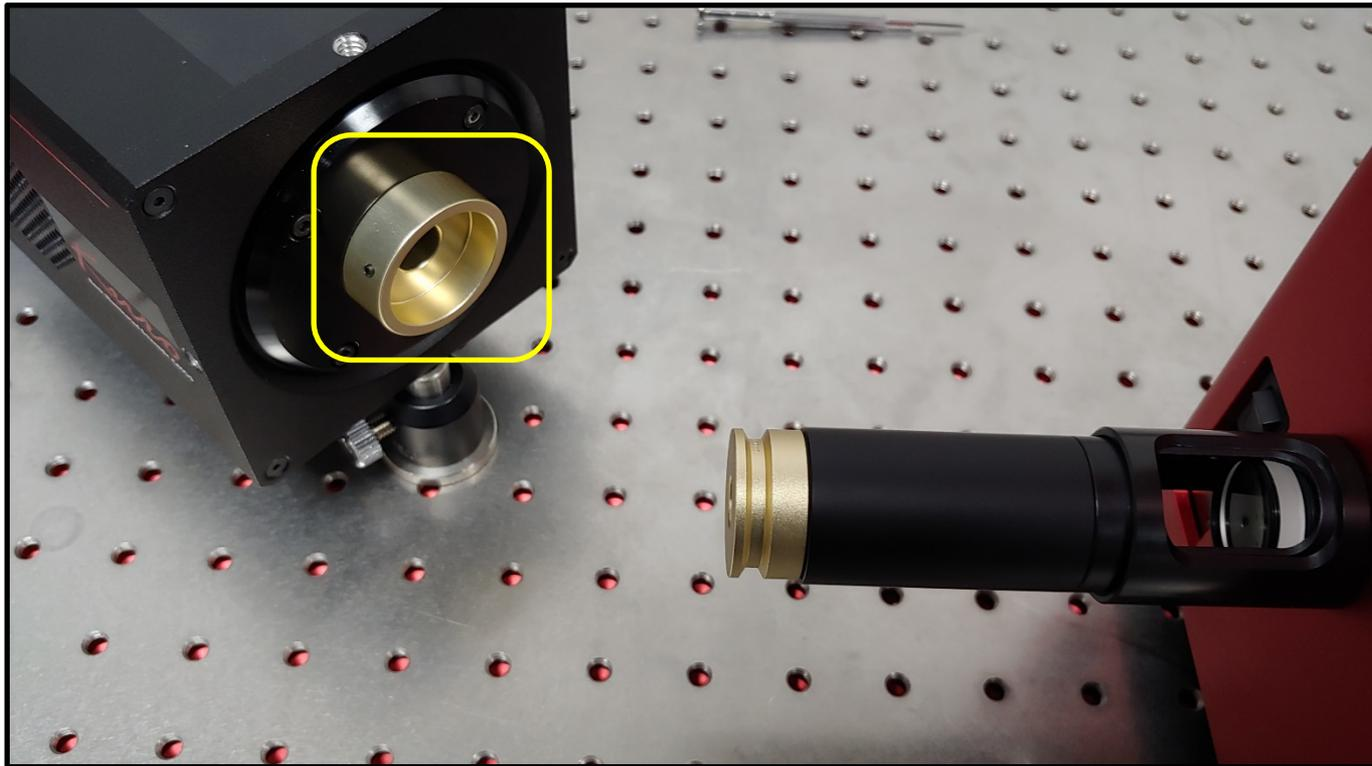
Assemble the provided **c-mount gold adapter** to the camera.
