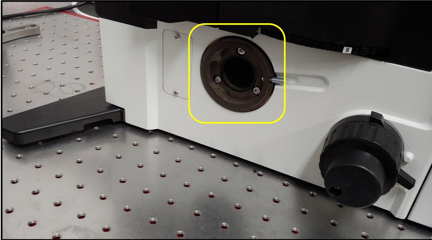
To convert your commercial fluorescence microscope into a hyperspectral imaging microscope, you need to attach FWS Poly into the emission port of your microscope. First, remove the camera attached at the emission port of your microscope
