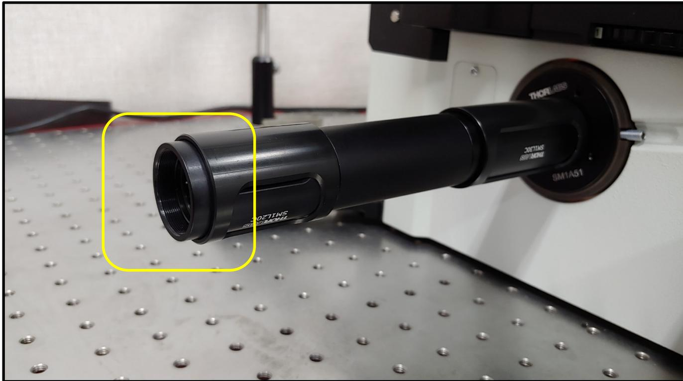
Then, screw in the **third lens tube**. The length of this tube is about 2 inches and contains a lens.
