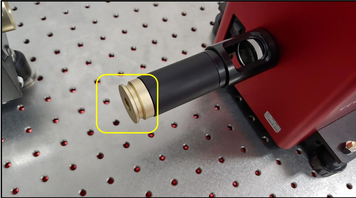
At the output port of the lens tube attach the gold adapter.
