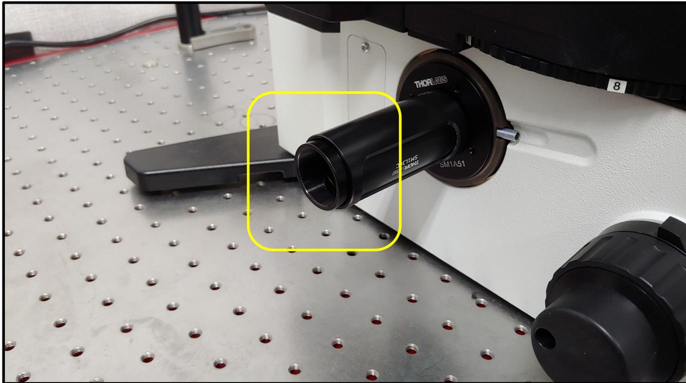
Then, screw in the **first lens tube** to the attached microscope adapter. The length of this lens tube will depend on the type of the user's microscope.
