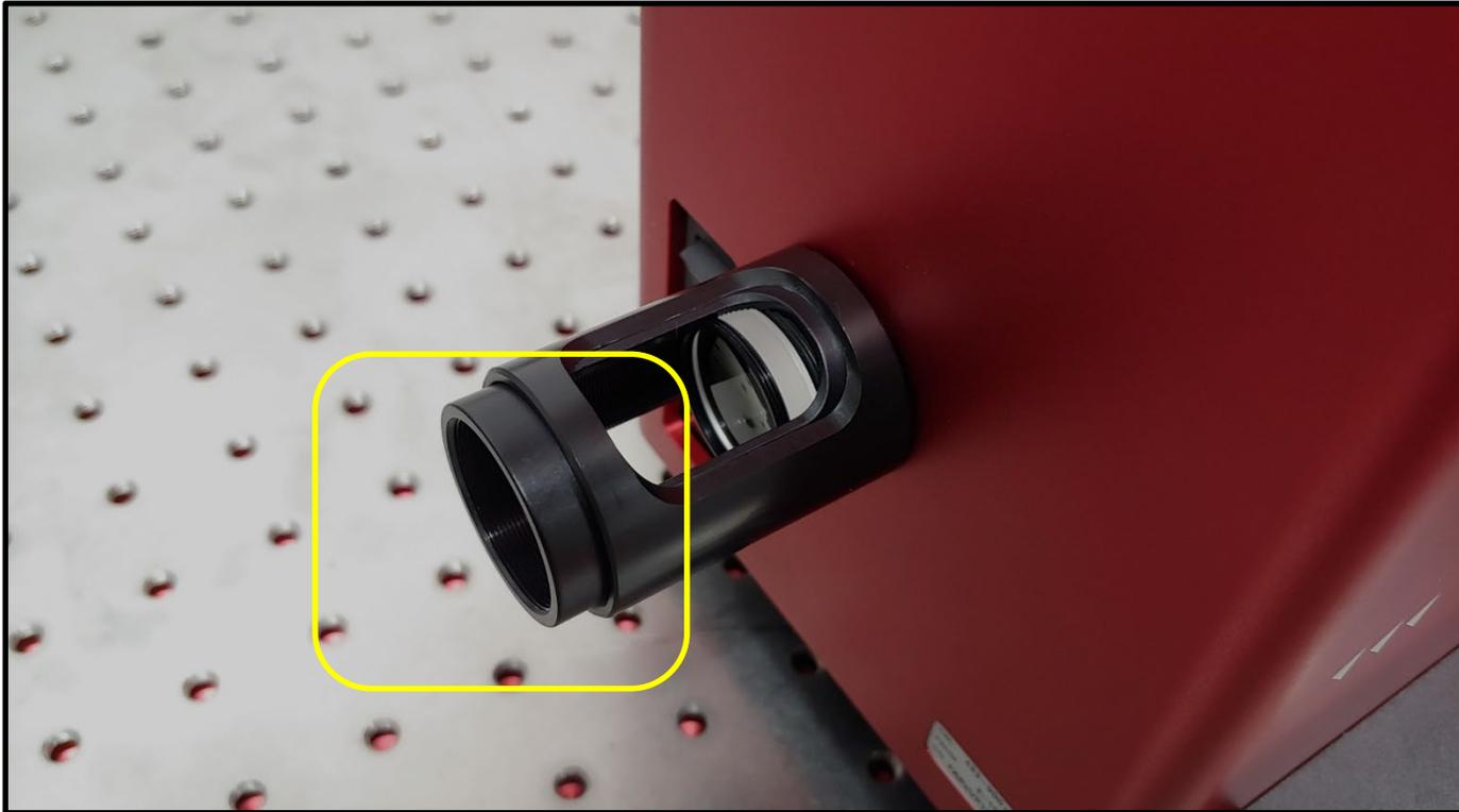
At the output port of FWS Poly attach the lens tube. This lens tube contains lens and is about 2 inches long.
